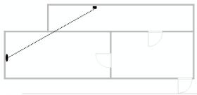
Simply by moving the Thermostat slightly to the right we have greatly improved the signal. The signal will now only travel through one internal wall
