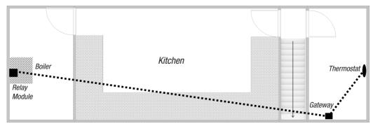
The above image shows the path that the signal will travel to communicate between the 3 units. This is an example of badly positioned items for the following reasons.
