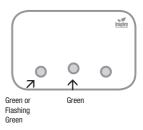
If there is no RF link displayed on the Thermostat, and it was switched on before the Gateway, it may take up to 10 minutes to link up. To avoid waiting, ensure the Gateway is plugged in, then reset the Thermostat by pressing and holding all four buttons for 5 seconds. The unit should reset and connect within 30 seconds.
