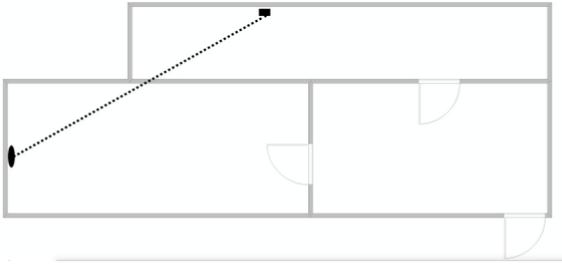
Simply by moving the Thermostat slightly to the right we have greatly improved the signal. The signal will now only travel through one internal wall
