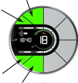
To reset the Ignite Wired Thermostat, press and hold the four highlighted buttons for 5 seconds.
